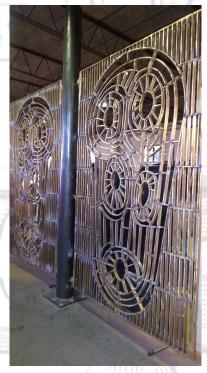
appointed by Laing O'Rourke to finalise the design details with Ian Simpson Architects, and fabricate two pairs of bronze gates for Mount Street. The gates were formed from bronze flats, TiG welded together.
