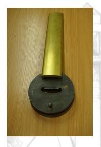
The works included the replication of hundreds of metres of new brass handrails to the stair cores and Shakespeare Hall. A metal die was made to allow for the correct profile to be produced by casting.
